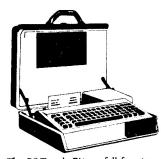
The PC Traveler™ is a full-function IBM-compatible, portable computer. A 28-pound wonder, it comes standard with a gas plasma display for 25 lines/80 characters, 128k RAM memory and an IBM PC-type removable keyboard. The dot matrix impact printer is bi-directional, 132 char-compressed.
